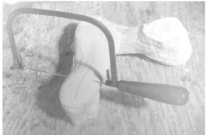
4 A 10pt. coping saw is a good tool to cut from the bottom of the cast down to the horizontal cut.
