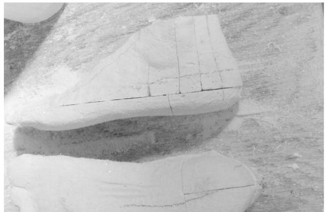
10 Aligning the heel parts to the marks on the side of the cast.
