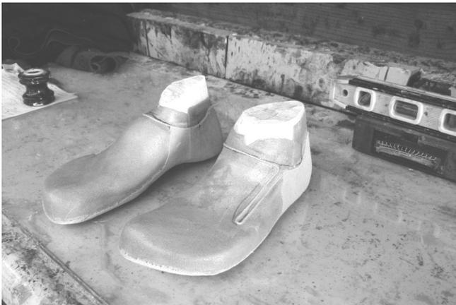
65 The inserts and lining have been added. The single knit sock has been added, latexed and the top front of the sock cut away. These are going to be soft shoes.
