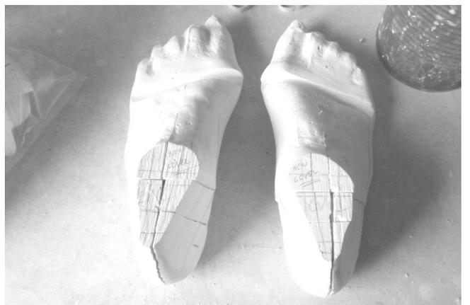
22 The casts are back together and the heels have been narrowed.
