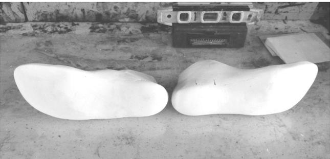
48 I have plastered the cast and transformed it into a "LAST".
